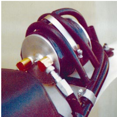
LEFT, BELOW LEFT & RIGHT: MAICO TEST BIKE WITH EARLY PROTOTYPE SHOCKS. NOTE THE TWO SHOCKS WERE CONNECTED TO A SHARED RESERVOIR MOUNTED ON THE REAR OF THE BIKE. THIS WAS AN EVALUATION VEHICLE FOR EARLY DESIGN IDEAS.
