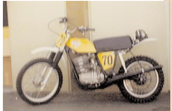
LEFT, BELOW LEFT & RIGHT: MAICO TEST BIKE WITH EARLY PROTOTYPE SHOCKS. NOTE THE TWO SHOCKS WERE CONNECTED TO A SHARED RESERVOIR MOUNTED ON THE REAR OF THE BIKE. THIS WAS AN EVALUATION VEHICLE FOR EARLY DESIGN IDEAS.
